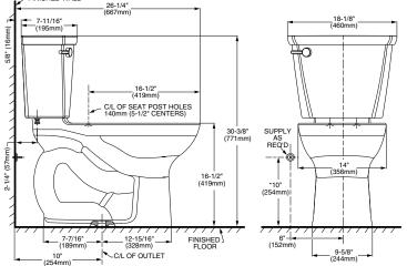
NOTES: THIS TOILET IS DESIGNED TO ROUGH-IN AT A MINIMUM DIMENSION OF 254MM (10") FROM FINISHED WALL TO C/L OF OUTLET. SUPPLY NOT INCLUDED WITH FIXTURE AND MUST BE ORDERED SEPARATELY. \* DIMENSION SHOWN FOR LOCATION OF SUPPLY IS SUGGESTED.
